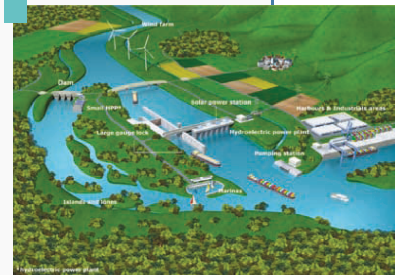
A typical CNR development scheme: 18 out of CNR's 19 hydropower plants have low heads. The low storage capacities of the reservoirs are used to modulate flow rates and thus optimise production.
